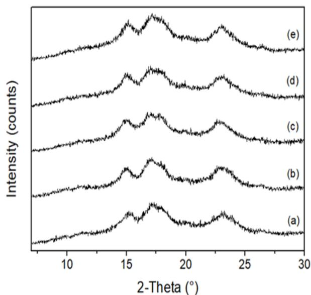
Figure 2. X-ray diffraction of (a) native starch, (b) ANN starch, (c) HMT starch, (d) ANN+HMT starch, and (e) HMT+ANN starch.
